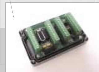
Clamp processor unit controls the clamping force applied to the paper roll. Advanced hydraulic and electronic features ensure minimized clamping force.
